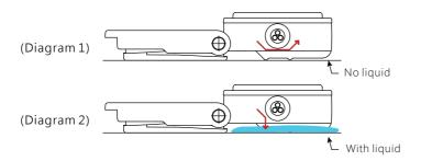
Diagram 1, the medium is air (no liquid). The light is completely reflected to the sensor.
