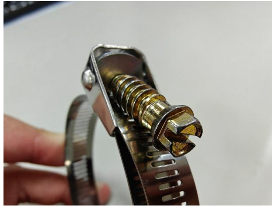
Step 3: Unfasten the locking screw and use a flat-blade screwdriver to tighten it
