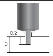
The sensor should be installed at a sufficient distance from the bends and cross-sectional points of the pipe to maintain accuspeed flow detection.
