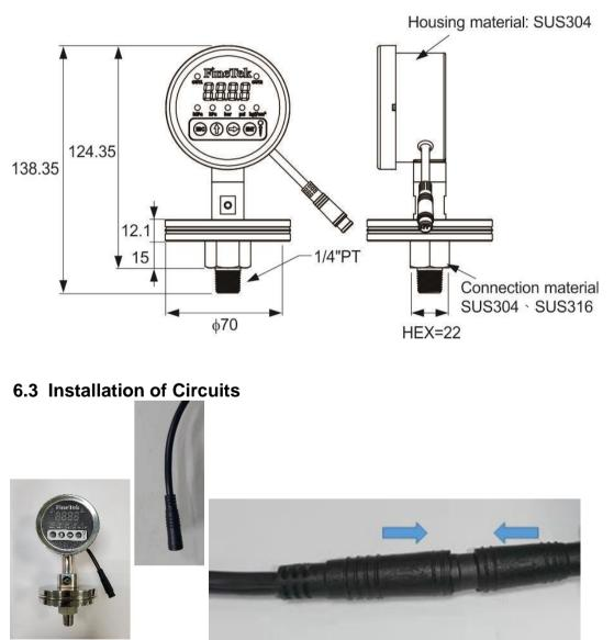
Once wiring is completed according to Section 5, finish installing the ECP pressure meter. Link and insert the quick joint of the cable in the arrow-indicated direction to complete installation of the circuit.
