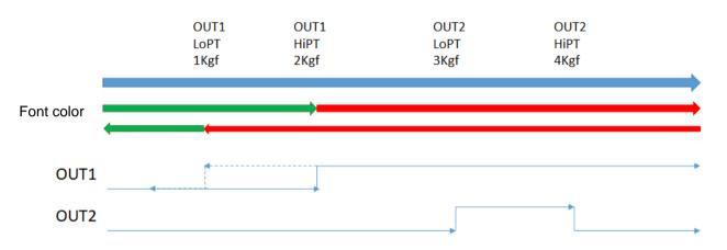
Once the measured pressure is greater than OUT2 LoPt 3 kgf/cm<sup>2</sup>, the On/Off joint OUT2 starts to act.
