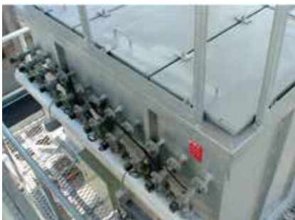
Dust collection machine uses the diaphragm valve to remove the cloth bag
