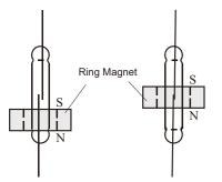
Reed switch open (OFF) Reed switch closed (ON)
