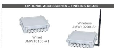
Finelink-RS485 collects data from 4 sensors, then transmit to receiver via cable or wireless solution. Each sensor has independent terminal block for wiring to prevent the failure of whole system, easy maintenance. Finelink-RS485 also provides the 24Vdc external power for 4 sensors.
