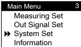
System Settings is provided to set System Language, Restore Default, Backlighting Setting, and LCD Contrast. Select System Setting in the Main Menu, and press button to edit the settings.
