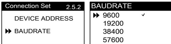
To connect with the computer successfully, it requires the same address of the device, which is 001 by default. Use and buttons to adjust the parameter value, and press button to confirm it.
