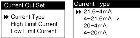
Press button in the Current Output Settings to enter Current Type Settings. A total of 4 current output types are available: 21.6mA~4mA, 4~21.6mA, 20~4mA and 4~20mA. Finally, press button to save.
