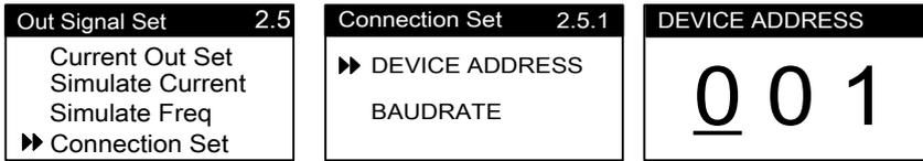
To connect with the computer successfully, it requires the same speed of the device, which is 9600bps by default. Use and buttons to switch between options, and press button to confirm it.
