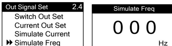
Press button in the Output Signal Settings to enter Simulated Frequency Output. Use and buttons to adjust the parameter value, and press button to save.
