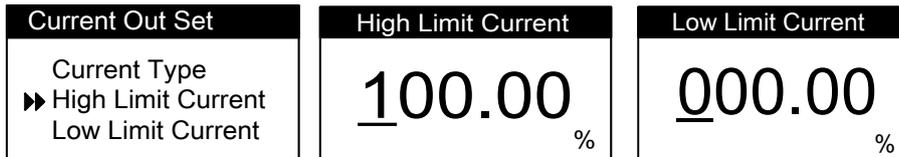
Press button in the Current Output Settings to enter Current Upper Limit or Current Lower Limit. Use and buttons to adjust the parameter value, and press button to save.
