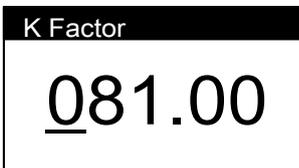
Use **▲** and **▶** buttons to adjust the parameter value, and press **ENT** button to confirm it.
