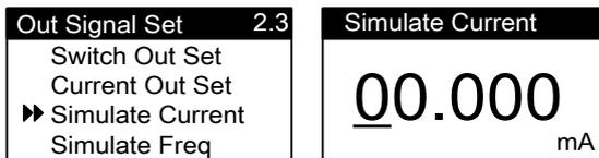
Press button in the Output Signal Settings to enter Simulated Current Output. Use and buttons to adjust the parameter value, and press button to save.
