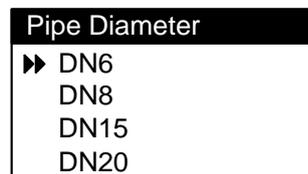
Use **▲** and **▶** buttons to switch, between the available options are DN6 · DN8 · DN8 · DN15 · DN20 · DN25 · DN32 · DN40 · DN50 · DN65, and press button to confirm it.
