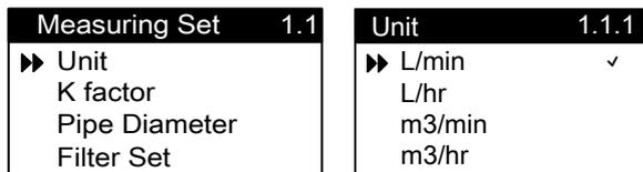
The measuring setting value can be in the unit of L/minutes, L/hour, m<sup>3</sup>/minute, m<sup>3</sup>/hour, gal/minute, gal/hour, kg/minute, kg/hour, ton/minute, and ton/hour. In the Measuring Set option, select Unit and press **ENT** button to enter the setting.
