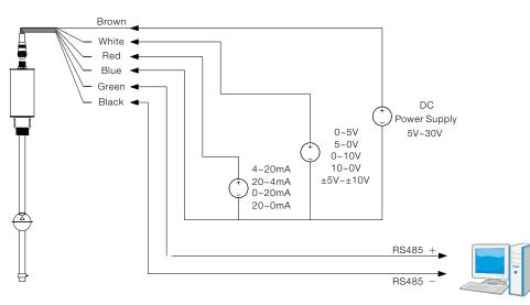
Total stem length= 500mm (Actual measurable length) + 73mm (S5 float)+15mm =588mm \* the float ball varies in size depending on different options.
