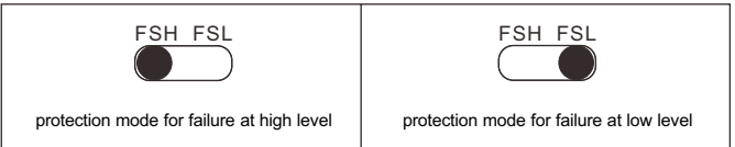
Fig-1 Failure-mode switch
