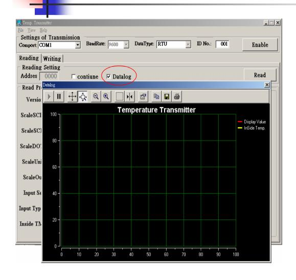
Click "Datalog" to checked(Pic B): it will apprear another window to show the curve of "Display value" & "Inside Temp."
